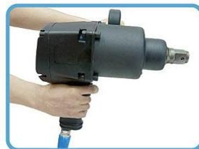
Press the trigger for running.
