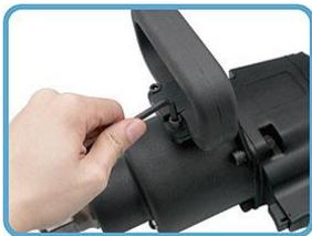
Use hex wrench turning clockwise to fix the screw which on the handle, and the handle will be fixed on the tool.
