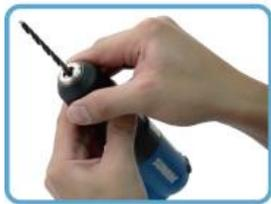
Holding the underneath piece of chuck and then clockwise the above piece in order to tighten the drill bit.
